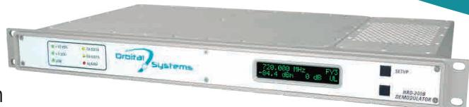
Orbital's HRD-200B high-rate demodulator is a versatile digital receiver used in the reception of standard EOS-DB Satellite formats, down-linked in X-band. This high-quality Quorum Communications Digital Signal Processing (DSP) demodulator provides repeatable performance, long-term operation without component drift, and flexible multi-mode operation for current and future satellite formats.
